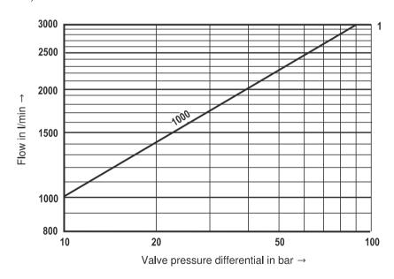
1 = Recommended flow limitation (flow velocity 30 m/s) in the valve connection bores
