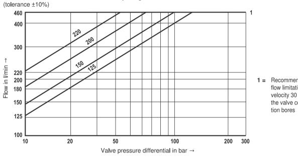
1 = Recommended flow limitation (flow velocity 30 m/s) in the valve connec-
